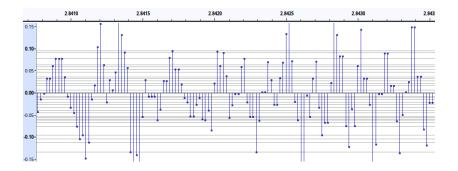
The vertical position of the wave can take any of the  $2^8$  = 256 values; 1 point = 1 byte.
